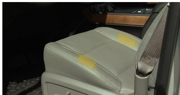
Figure 7. General Motors Safety Alert Seat Vibration Areas (in yellow) [13]
