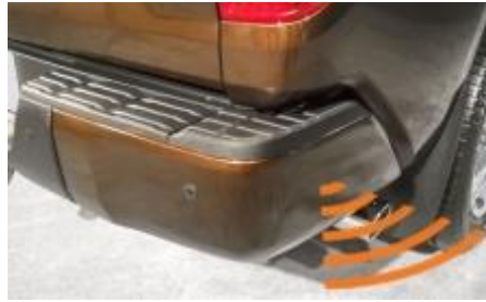
Figure 3. Bumper Blind Spot Sensors on a 2015 Toyota Tundra [6]
