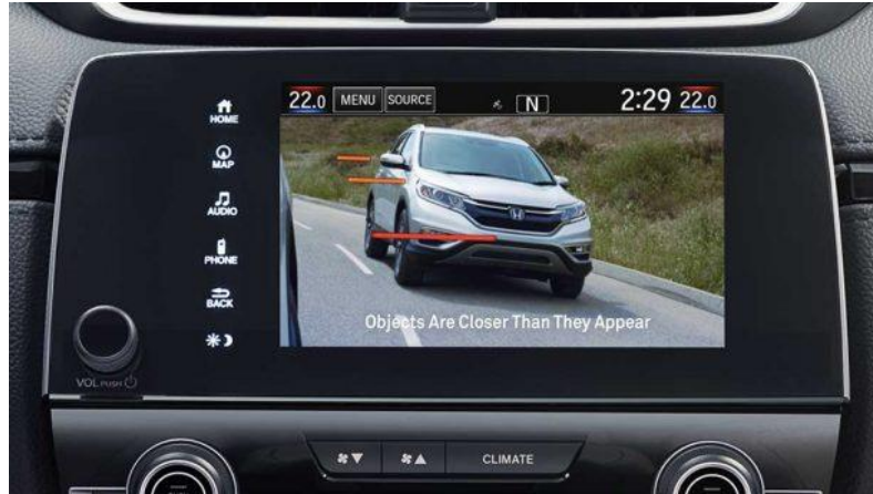
Figure 5. Honda Display Showing Possible Impact Areas of your Rear Bumper [8]
